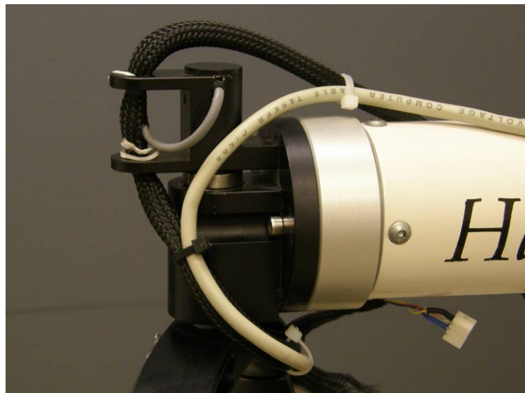
Figure 3 Robot end-effector force sensor. One of gimbal potentiometers is partially also visible.
